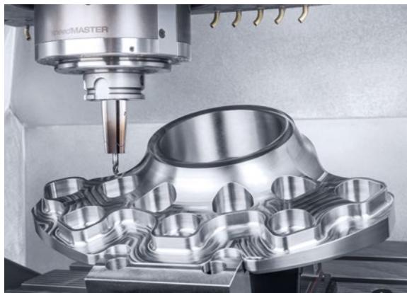
2: Motor spindle SK 40 20,000 rpm 130 Nm | 35 kW (40% DC)
